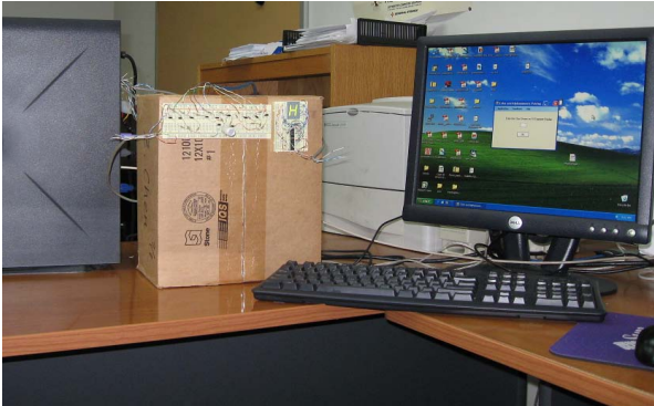
Fig. 2. Overall Experimental Setup of the Color and Alphanumeric Pairing (the cardboard box with the multi-color LED and the SSD, simulates, e.g., an access point in a cyber-cafe; the desktop simulates the laptop.)
